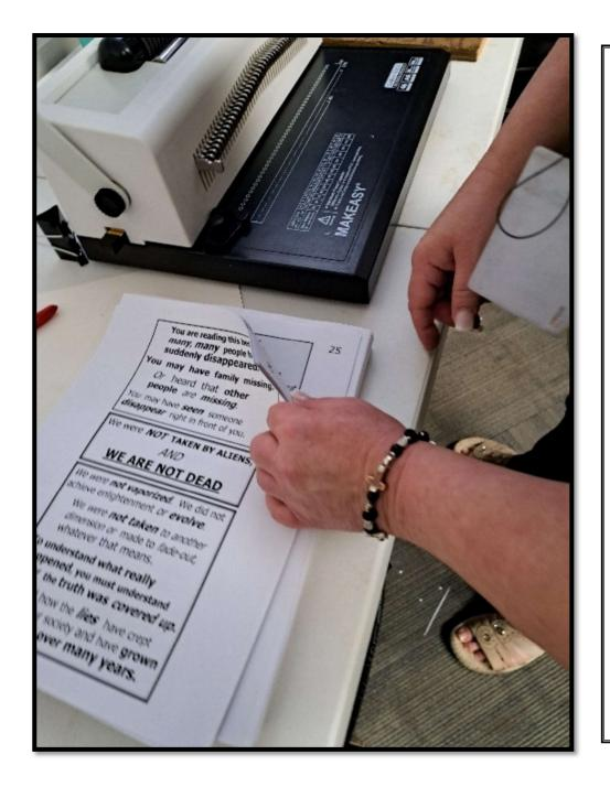
We punch approximately 10 -12 sheets at a time. Punching too many pages at a time can make the holes misalign. Plus it's difficult punch through the paper to make the holes if you're trying to do too many at once.
