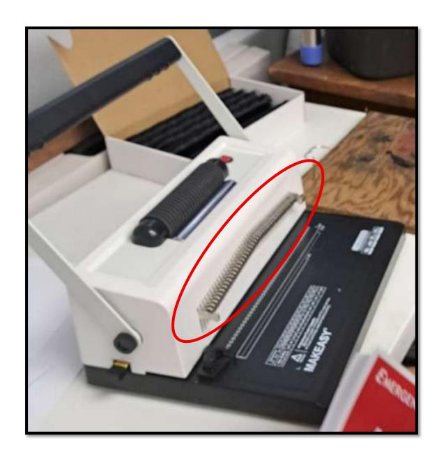
These PINS adjust how many and how far apart the holes will be punched.
