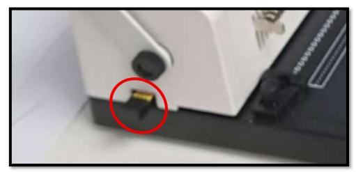
This little lever on the left side of the machine determines how far the hole will be punched from the edge of the paper. We put this on the farthest 'outside' setting. Pulled out as far as it will go, which places the holes further onto the pages.
