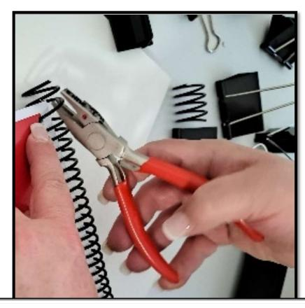
Holding the pliers and the book exactly as indicated in this picture (from the upper right corner), works best. Snip and bend to prevent the coil from coming back through the holes.
